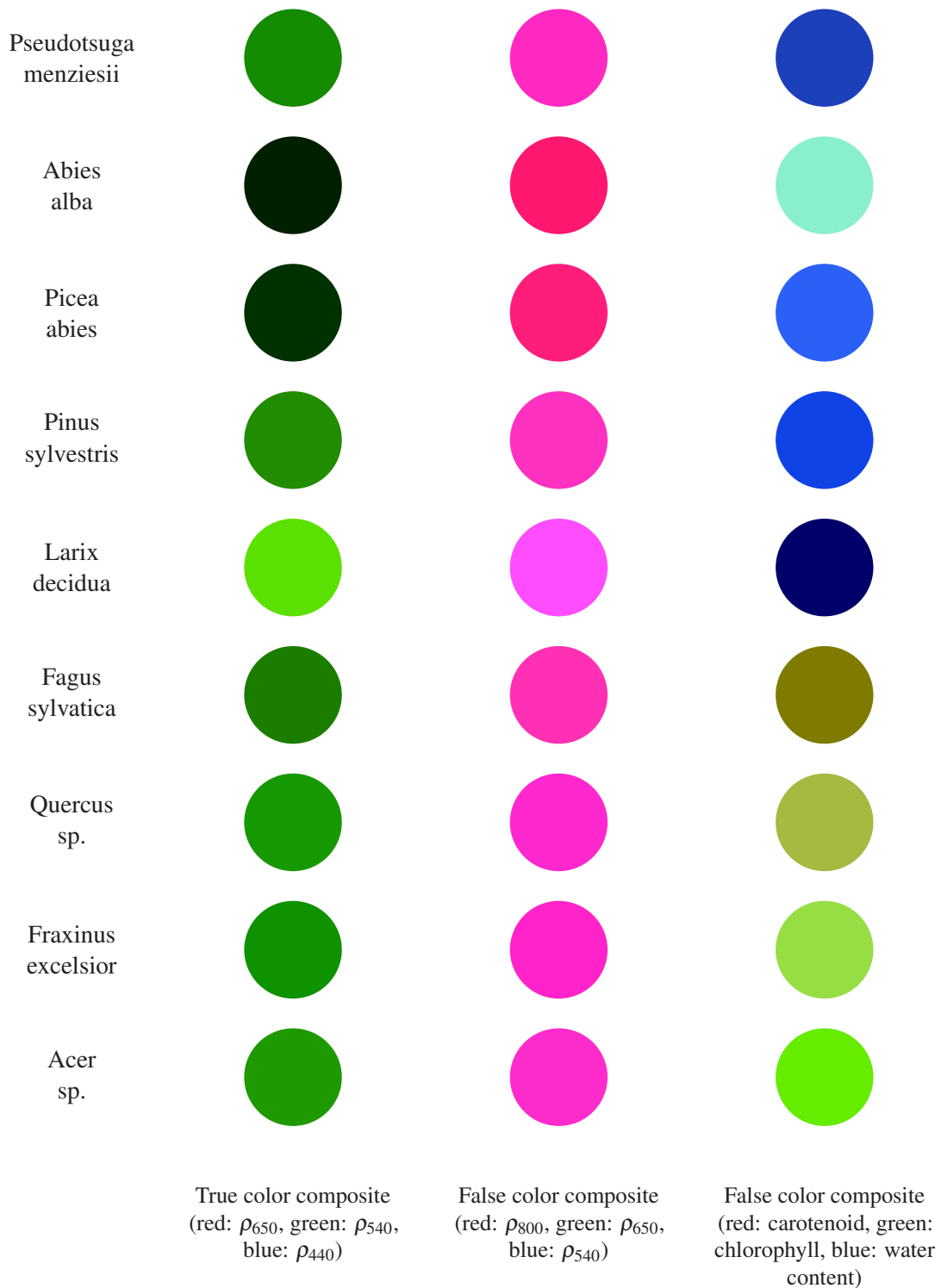
Figure 5.8: Three different color composites for nine selected tree genus/species (mixed age classes) obtained with the APEX sensor in July 2014. The colors are based on the median values of pixels with a class purity above 85%. The last color composite (on the right) combines an estimation of carotenoid content CAR = (\rho_{515}^{-1} - \rho_{565}^{-1}) \cdot \rho_{780} , chlorophyll content CHL = (\rho_{550}^{-1} - \rho_{780}^{-1}) \cdot \rho_{780} and water content W = 1 - \frac{\rho_{1193}}{\rho_{1126}} (cf. Gitelson et al. (2006); Schneider et al. (2017)).
