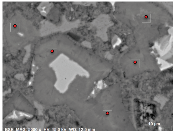
Figure 2.4 EDS point analysis of inner C-(A)-S-H
