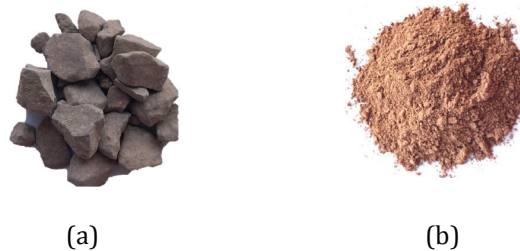
Figure 5.2 Visual observation of the raw clays for (a) rotary kiln and (b) fluidized bed
