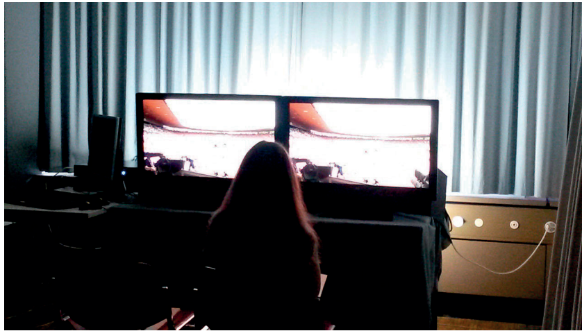
(b) 2000 nits Maui monitors, set at 1000 nits. This SDR pictures hardly represent the DR rendered on HDR displays, this explains that bright parts of the content seem burnt
