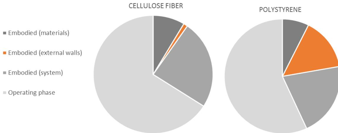
Figure 11: Percentage distribution of impacts on GWP indicators for macro-components. The analysis is made for case 60 in the first sensitivity analysis (identified as the best case), changing only the insulation materials: cellulose fibre and polystyrene
