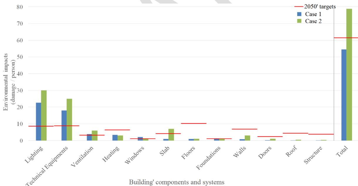
Figure 2 : Comparison of the impacts of building components and systems with their respective targets (red lines)
