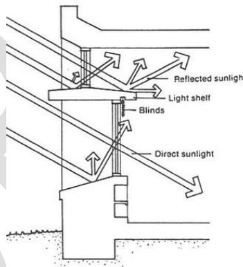
Figure 15: Scheme showing the functioning of the light shelves to bring light deeper inside the room
