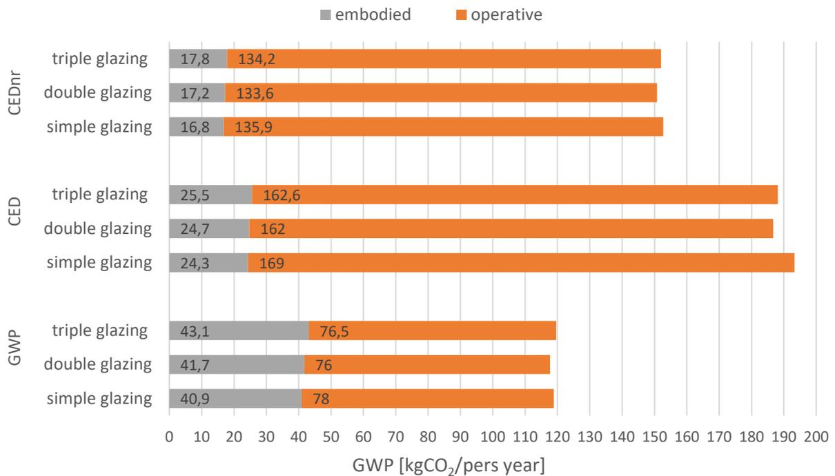
Figure 12: Operating and embodied impacts for carbon emissions in a case study with three different scenarios: single-glazed ( $U: 6W/m^2K - g: 0.92 - t: 0.83$ ), double-glazed ( $U: 1.1W/m^2K - g: 0.62 - t: 0.8$ ) and triple-glazed ( $U: 0.7W/m^2K - g: 0.5 - t: 0.72$ ) windows. Windows to wall ratio: 0.5 - Frame 25% wood
