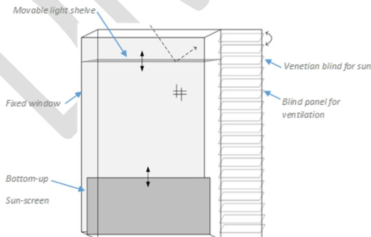
*Figure 14: Sketch of the “climate box” element of the solution – transparent components with shading system, light shelves and a special panels for ventilation*
