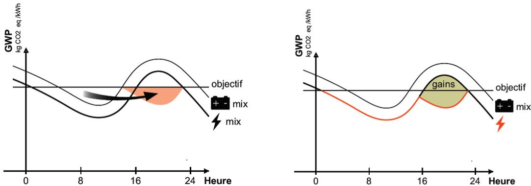
Figure 23: Concept of decarbonisation of electricity from the grid. In a first step, the low-carbon electricity is stored (left side) to be used when the carbon content of the electricity of the mix reaches a higher level than that of the stored electricity (right side).
