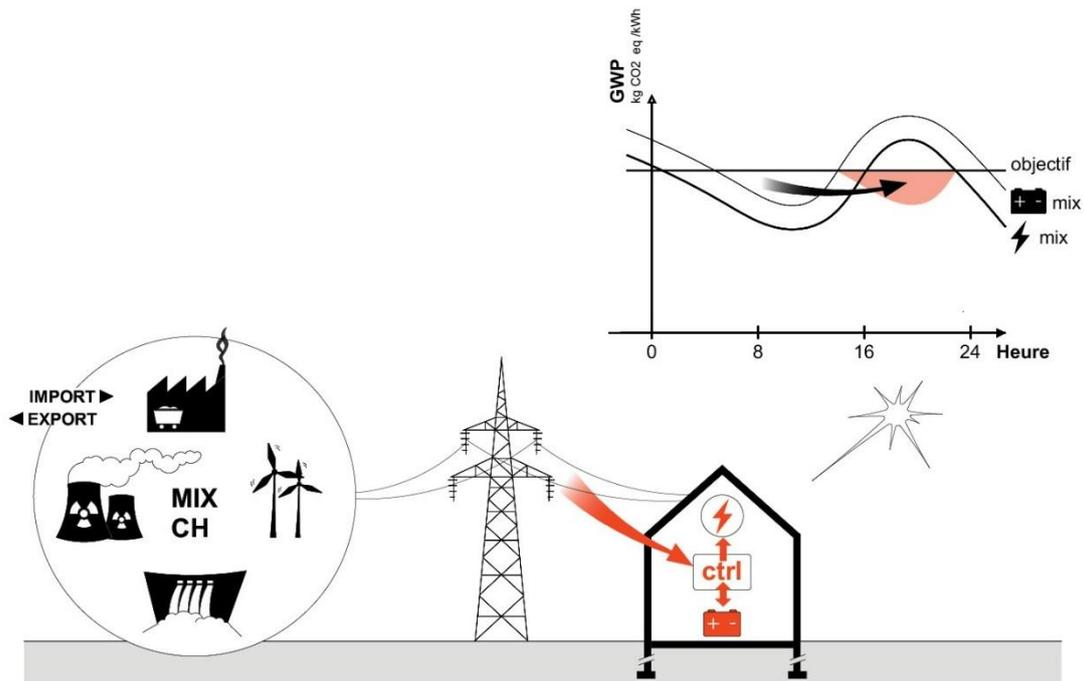
Figure 19: Temporal variation of the carbon content of the electricity mix and the possibility to integrate storage for a better correlation between low carbon electricity and its consumption
