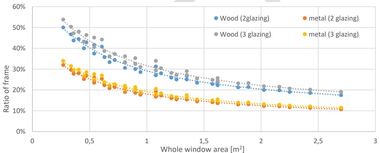
Figure 13: Relationship between the whole window area and the percentage of frame for two different profiles (wood and metal) and for different kinds of panes
