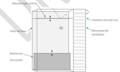
Figure 14: Sketch of the "climate box" element of the solution – transparent components with shading system, light shelves and a special panels for ventilation
