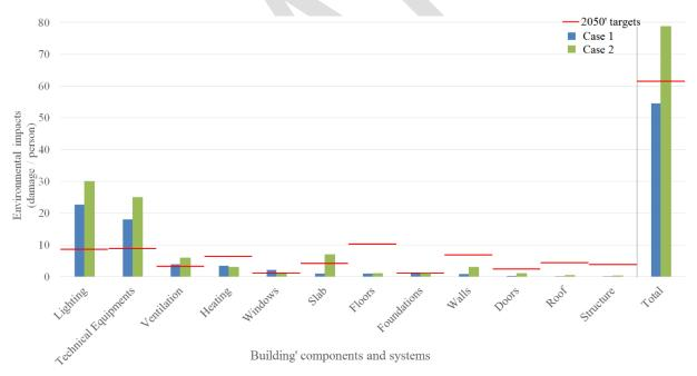
Figure 2 : Comparison of the impacts of building components and systems with their respective targets (red lines)
