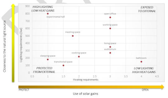
Figure 29: Layout of user spaces in relation to lighting/thermal requirements
