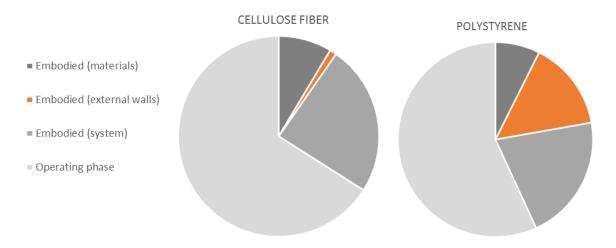
Figure 11: Percentage distribution of impacts on GWP indicators for macro-components. The analysis is made for case 60 in the first sensitivity analysis (identified as the best case), changing only the insulation materials: cellulose fibre and polystyrene
