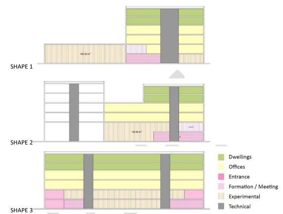
Figure A 15: The three different geometrical solutions proposed for the smart living lab
