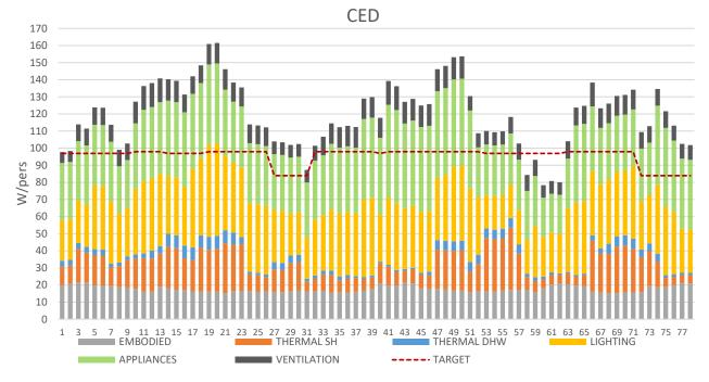
Figure A 1: CED Index for the 78 simulations of SA I
