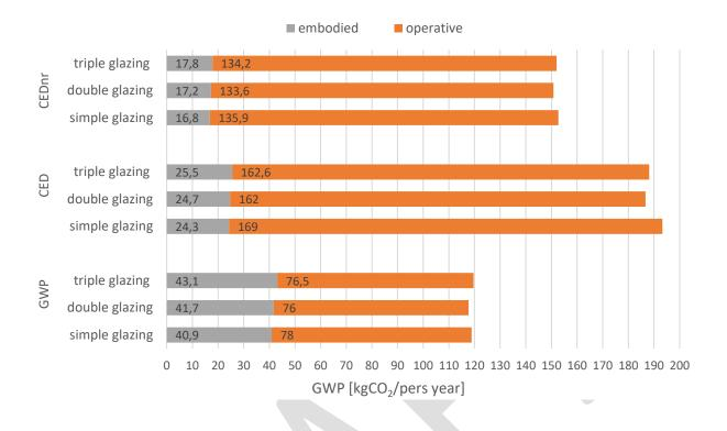
Figure 12: Operating and embodied impacts for carbon emissions in a case study with three different scenarios: single-glazed (U:  $6W/m^2K$  - g: 0.92 - t: 0.83), double-glazed (U:  $1.1W/m^2K$  - g: 0.62 - t: 0.8) and triple-glazed (U:  $0.7W/m^2K$  - g: 0.5 - t: 0.72) windows. Windows to wall ratio: 0.5 - Frame 25% wood
