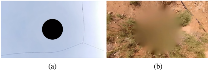
Fig. 4: Examples of post-processing on the poles due to missing areas: (a) a black circle and (b) a (inpainted) blurred circle.
