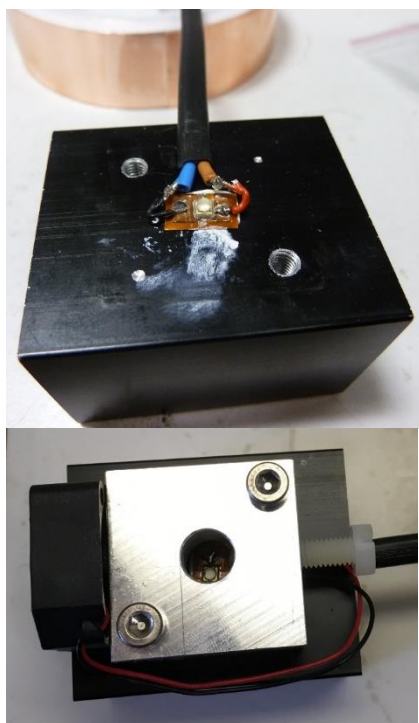
Figure S15. Finished lighting source without (top) and with (bottom) aluminium housing.
