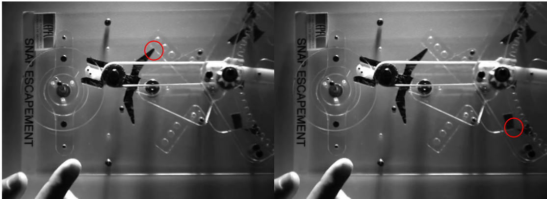
Figure 5.33 – Unlocking of the escape wheel
