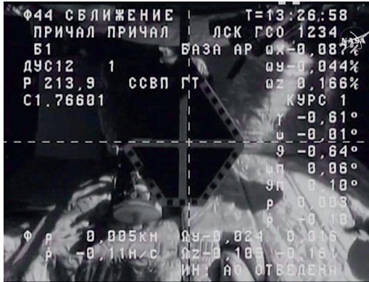
Figure 4.8 – Circular pattern with out-of-plane marker used for the Soyuz and Progress docking monitoring. Credit: NASA.
