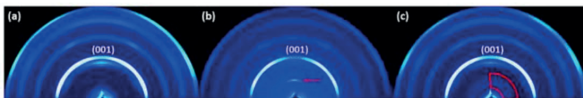
Figure 74. 2D GIWAXS images of (a) HT-ZnPc (b) HBT-ZnPc and (c) TB-ZnPc. GIWAXS samples were prepared with similar procedures as device fabrication. Doped with LiTFSI, FK209 and TBP, HTMs were spin-coated on the underlying perovskite film.
