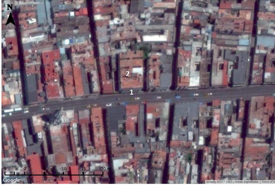
Figure 3.1: Data collection site (Simon Bolivar Street). 1: Thermo-Scientific ADR 1500 profiler and traffic video recording. 2: AIRDAM anemometer. Adapted from Google Earth.
