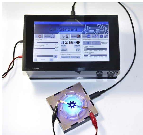
Fig. 10. PPV in standalone configuration with Raspberry Pi, 7" touchscreen and battery. PPV is pictured driving a DEA mounted on a strobe light. PPV provides power to the light, as well as a logic signal synchronized with the high voltage square signal driving the actuator.
