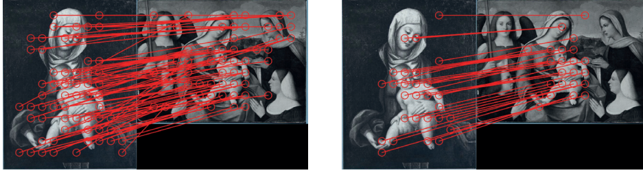
Figure 3.22: Example of using the CNN feature maps to match images. Left: candidate matches computed from the CNN descriptors (each cell of the feature map). Right: resulting matches based on spatial filtering.
