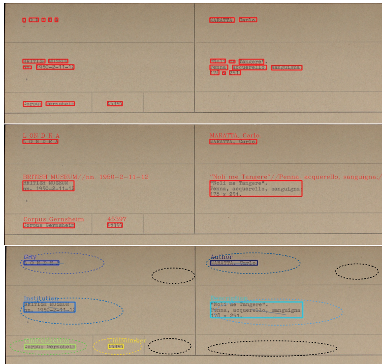
Figure 2.13: Words are detected, then clustered in paragraphs before being assigned to their corresponding label with the layout model.
