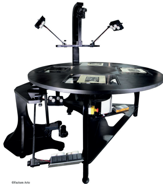
Figure 2.3: The designed scanner. Notice the two cameras for simultaneously digitize the two side of the document, and their respective sets of flashes.
