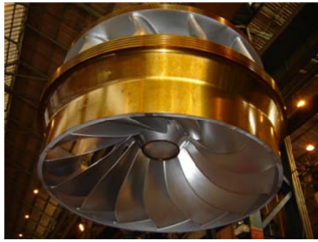
b) New Francis turbine runner of Unit #3
