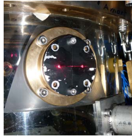
Fig. 9: Draft tube cone alignment check
