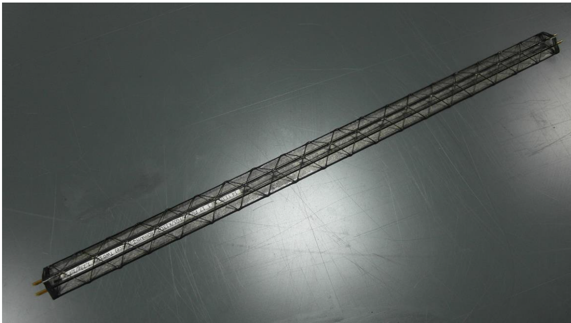
Figure 1. One of the ultra-lightweight carbon fiber support structures with integrated cooling system.
