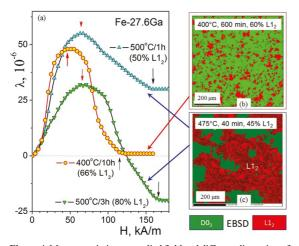
Figure 4. Magnetostriction vs applied field and different dispersion of the L1, (red color) phase at 400 (fine) and 475/500°C (coarse grains).
