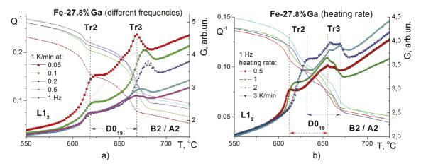
Figure 6. Second and third transition peaks in the Fe-27.8Ga sample: a) influence of the frequency of vibrations (from 0.05 to 1 Hz, heating rate 1 K/min), b) influence of the heating rate (from 0.5 to 3 K/min, 1 Hz).
