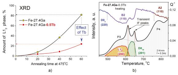
**Figure 7.** (a) Amount of L1<sub>2</sub> phase determined by X-ray analysis after isothermal annealing in the Fe-27.4Ga (yellow circles) and in the Fe-27.4Ga-0.5Tb (red circles) samples; (b) Phase transitions in the Fe-27.4Ga-0.3Tb sample according to the *in situ* neutron diffraction (Intersity, left Y-axe) and TDIF (black curve corresponds to right Y-axe).
