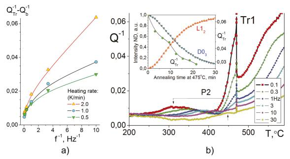
**Figure 3.** a) The Tr1-peak height as a function of inverse frequency for three different heating rates; b) TDIF curve with interrupted heating at 470°C. Inset: The decrease of the Tr1 peak as a function of time of isothermal annealing (green circles) and intensities of neutron diffraction lines from decaying D0, phase (blue down triangles) and growing L1, phase (red up triangles) under the same conditions.
