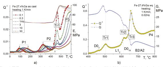
Figure 1. TDIF curves measured at heating with 1 K/min rate using bending (up to 600°C, DMA Q800; left figure) and torsion (up to 800°C, inverted pendulum; right figure) vibrations with different frequencies from 0.02 to 30 Hz (see in figures).
