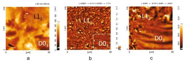
**Figure 5.** Topography (a), low magnification MFM (b), and high magnification MFM (c) images of the Fe-27.8Ga sample annealed at 400 °C for 600 min showing  $DO_3$  (darker contrast) and  $L1_2$  (brighter contrast) phases.
