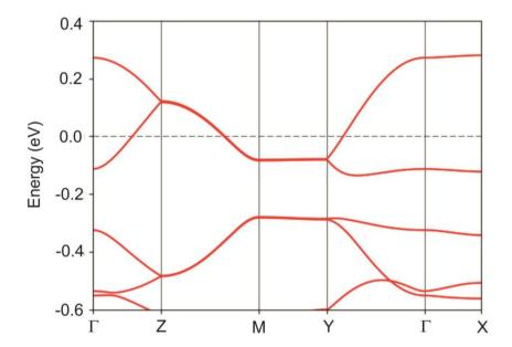
**Figure 4.** (Color online). Calculated band structure for the 300 K crystal structure of κ-ET-Cu. The energy zero corresponds to the Fermi level.  $\Gamma = (0,0,0)$ , X = (1/2,0,0), Y = (0,1/2,0), Z = (0,0,1/2), and M = (0,1/2,1/2) in units of the reciprocal lattice vectors.
