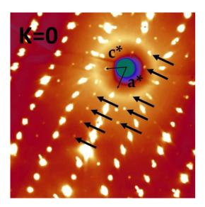
**Figure 1.** (Color online). Reconstruction of the ( $\mathbf{a}^*$ ,  $\mathbf{c}^*$ ) reciprocal plane taking into account the absorption correction. The thin arrows indicate the directions of the reciprocal lattice parameters, and the thick arrows show the reflections forbidden in the P2<sub>1</sub>/c space group.
