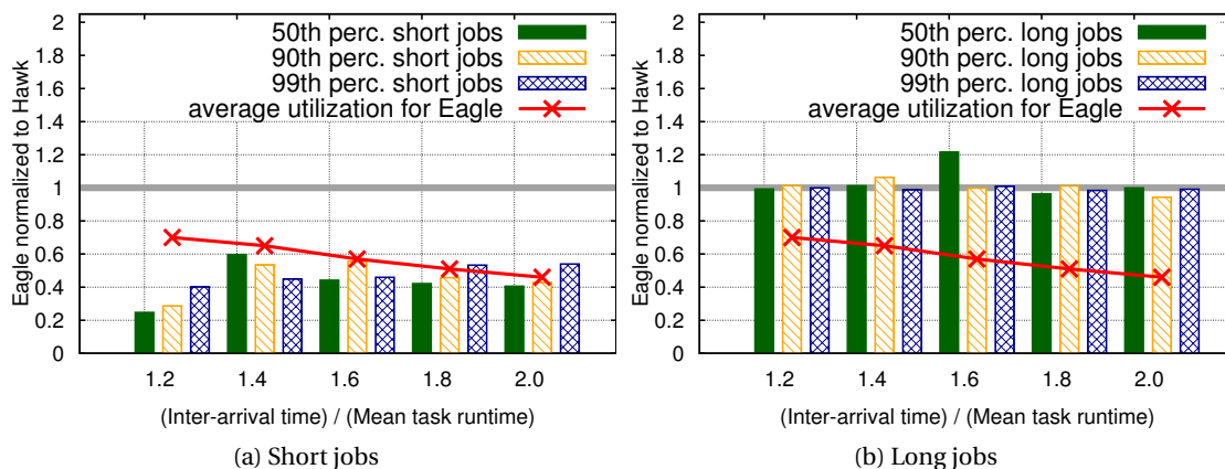
Figure 3.9 – 50/90/99th percentiles of the job completion times in Eagle, normalized to Hawk for a 3300-job sample of the Google trace.
