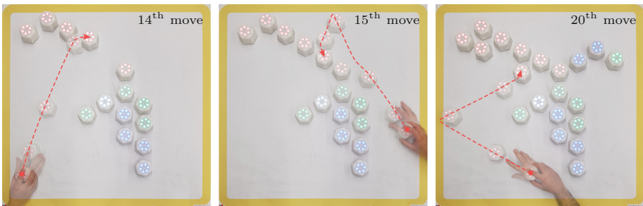
Fig. 1. Bubble shooter game with Cellulo platform [3] where the goal is e.g. to build the largest group of the same color. Launched robots collide elastically with existing robots (all 3 figures) and the walls (middle and right) before stopping.
