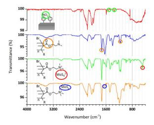
**Figure 2.** FTIR spectra of the MoS<sub>x</sub>/polymer brush composite at different stages of fabrication. The corresponding chemical structure is drawn for reference. The circled features on the spectra
