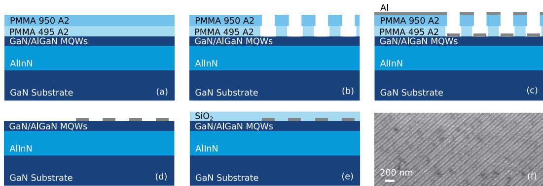
Figure 4.2 – Fabrication of metal grating couplers. (a) A PMMA double layer is spin coated onto the sample. (b) The resist is exposed using e-beam lithography and subsequently developed. The PMMA 495 layer has a lower dose threshold, which results in an undercut under the top PMMA 950 layer. (c) The Al film is deposited onto the sample using e-beam evaporation. Due to the undercut in the PMMA double layer, the parts of the Al film in the regions of exposed PMMA are not connected to the rest of the film and will not be affected by its lift-off. (d) The PMMA layer is lift-off with the superfluous Al in acetone at 37°C. (e) The SiO 2 top cladding is deposited. (f) Scanning electron micrograph of the Al grating coupler after lift-off, corresponding to (d).
