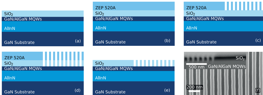
Figure 4.1 – Fabrication of dielectric grating couplers. (a) A 100 nm thick SiO 2 layer is deposited on the III-N structure by PECVD. (b) A ~100 nm ZEP resist layer is spin coated on the sample. (c) The resist is exposed using e-beam lithography and subsequently developed. (d) The grating pattern is etched into the SiO 2 layer using ICP RIE. (e) The resist layer is removed using an oxygen plasma. (f) SEM image of the dielectric grating coupler after etching, corresponding to (d). The main image shows the top view, while the inset shows a tilt-corrected cross-section view after focused ion beam milling.
