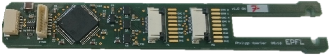
Figure 5.4: Picture of the integrated drive electronic for the 25mm prototype
