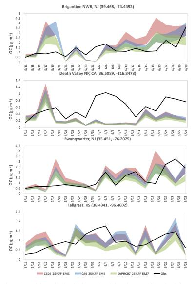
Figure 7. Time-series plots of IMPROVE OC vs. simulated OC at selected sites from sensitivity simulations of different gas-phase mechanisms. The colored bands represent the range of OC values for ratios 1.4 to 2.1.
