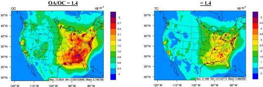
Figure 2. Overlay of obs data (markers) vs. sim data (background) for IMPROVE OC and STN TC and for OA / OC ratios of 1.4 and 2.1 for the case CB05\_25%FF\_EM3.
