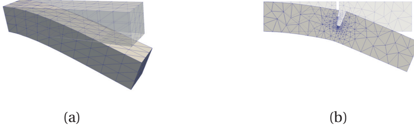
Figure 5.1 – (a) initial condition and a snapshot of the 3D beam. (b) initial condition and a snapshot of the 2D beam with a cavity.
