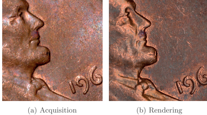
Figure 3.3: BRDF acquisition and rendering: (a) a close-up of a US penny under a specific illumination and (b) a rendering of the same coin under a different artificial illumination.
