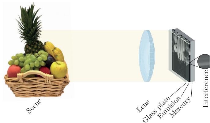
Figure 4.1: Principle of Lippmann photography: the scene on the left is focused with a photographic lens on the plane of the emulsion. At the back of the emulsion is a mercury layer; when the light field hits the mercury layer, it reflects, and interferes with itself. Its spatially varying intensity creates patterns that are captured inside the depth of the emulsion (see the close-up).
