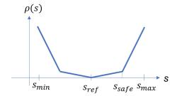
Figure 2: Terminal cost on state of charge. It is designed to favour SoC close to the reference with piecewise affine shape penalizing strongly SoCs close to the maximum and minimum allowed SoCs.
