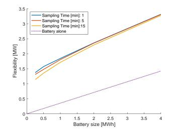
Figure 6: Maximum flexibility that can be offered as a function of battery size.
