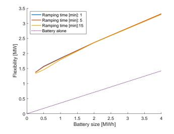
Figure 9: Maximum flexibility that can be offered as a function of battery size.
