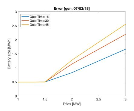
Figure 5: Minimum battery storage capacity size required as a function of flexibility offered and gate closure delay time.
