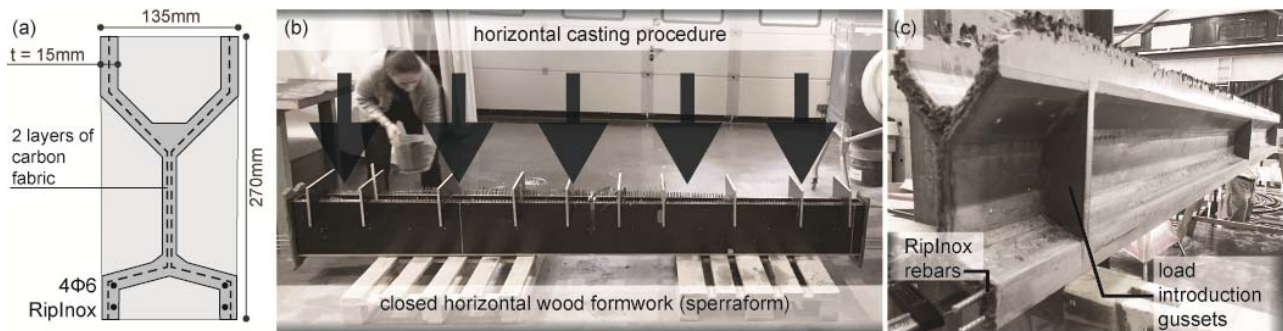
Figure 6. X-Beam: (a) cross-section; (b) casting procedure; (c) final result after demoulding.
