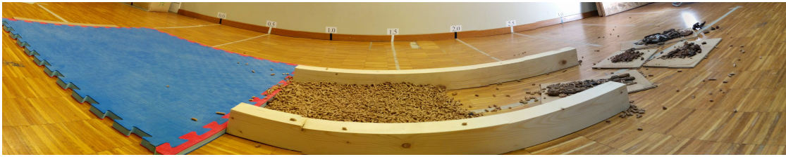
Figure 9.25 – Rough terrain setup for Oncilla; Locomotion direction: parquet, two stairs up of 0.010m and 0.015m , rough tatami, step down into pebbles and fixed wooden obstacles (maximum height: 0.03[m] ( \approx 16\% of the leg length) between footholds
