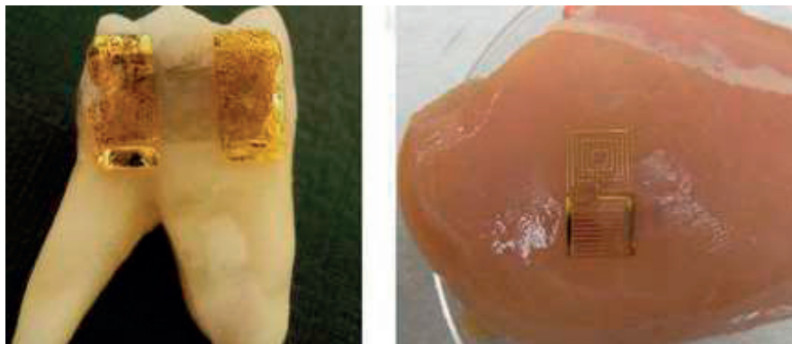
Figure 2.4 Examples of wearable sensors for saliva sampling. Adapted from [70].
