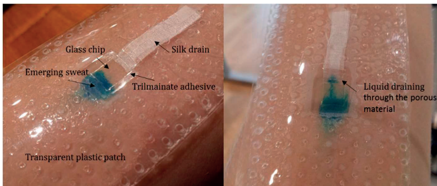
Figure 4.5 Left. Microfluidic collection device for high sweat rates. Right. After 15 minutes of sport, sweat started to get drained by the absorbent material
