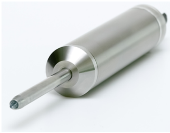
Fig. 5: The fast temperature sensing module. It is 20 cm long and 2.5 cm in diameter.
