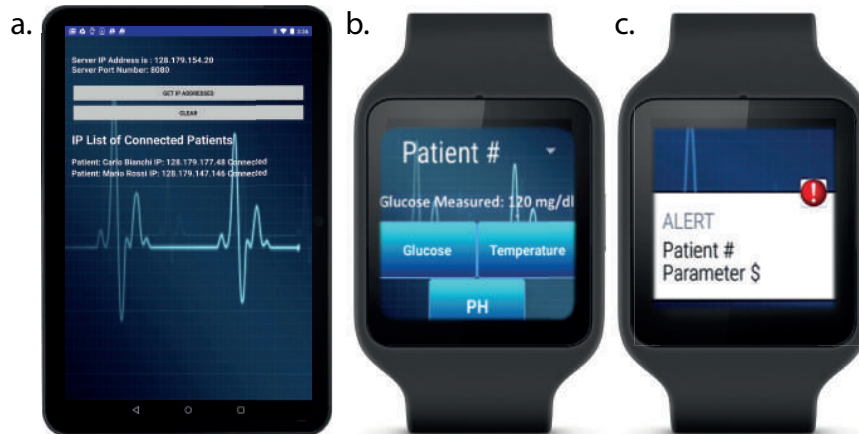
Figure 6.5 – a) Server Android application: it keeps track of all the patients connected to the network and enables the bidirectional communication between them and the smart-watch. Smart-watch Android Wear application: b) the doctor can query for specific parameters from a connected patient, and c) is alerted in case of out-of-safe-range measured parameters.
