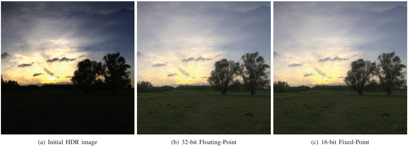
Fig. 5: Initial 1024 \times 1024 HDR image (a) and tone-mapped versions obtained using either floating-point (b) or fixed-point (c) Gaussian blur accelerators.
