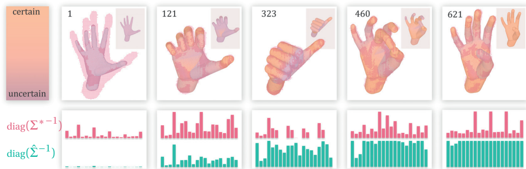
Figure 4.1 – Our adaptive hand tracking algorithm optimizes for a tracking model on the fly, leading to progressive improvements in tracking accuracy over time. Above: hand surface color-coded to visualize the spatially-varying confidence of the estimated geometry. Insets: color-coded cumulative certainty. Notice how in the last frame all parameters are certain. Below: histograms visualize the certainty of each degree of freedom, that is, the diagonal entries of the inverse of the covariance estimate from: (a) data in the current frame \Sigma^* , or (b) the information \hat{\Sigma} accumulated through time by our system.
