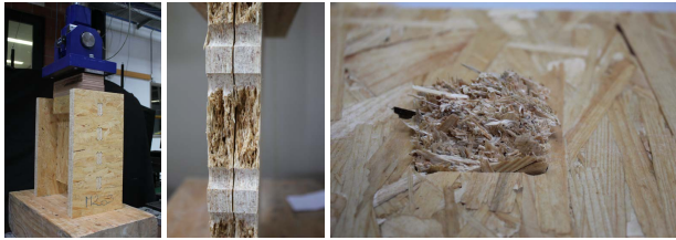
Figure 3: (a) Experimental Setup (b) Failure mode, web part (c) Failure mode, flange part
