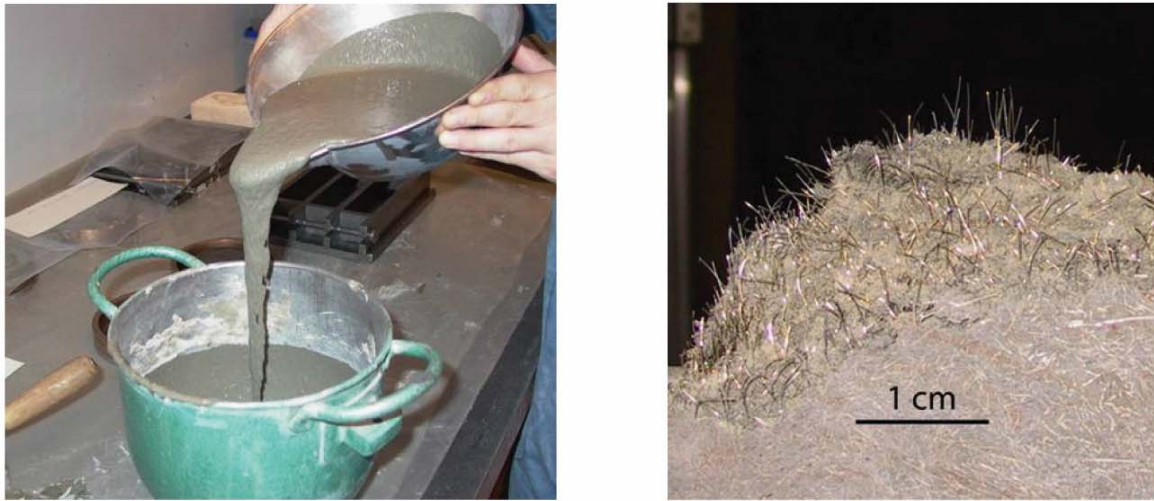
Figure 4-1: a) UHPFRC at fresh state (mix CM1) and b) texture of the hardened material CM2 shown on a fracture surface.
