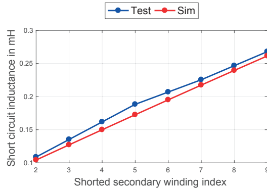
Figure 9.12 Short circuit inductances with W_{s1} supplied and one of the other W_s s shorted
