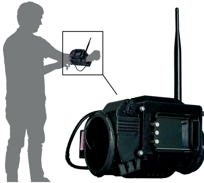
Figure 6.8 – The long range communication system. The 3D printed enclosure contains Odroid-C1+ with a touchscreen and three tactile buttons, XBee module with an antenna and a battery. Although bulky, the system can be carried around a wrist.
