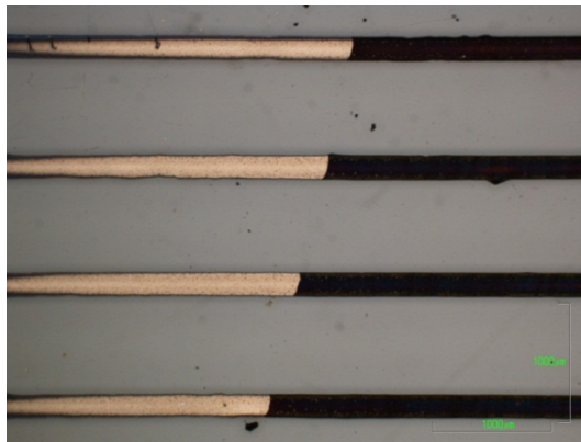
Fig 19: Ag/AgCl electrodes (right, dark colour) formed after chemical treatment with \text{FeCl}_3 over Ag lines (left)
