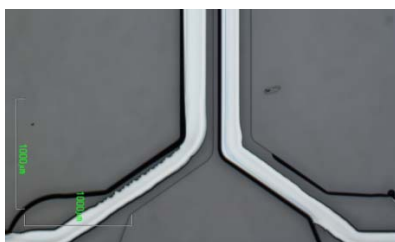
Fig 26: Ag line touching the wall of the microchannel compromise its conductivity
