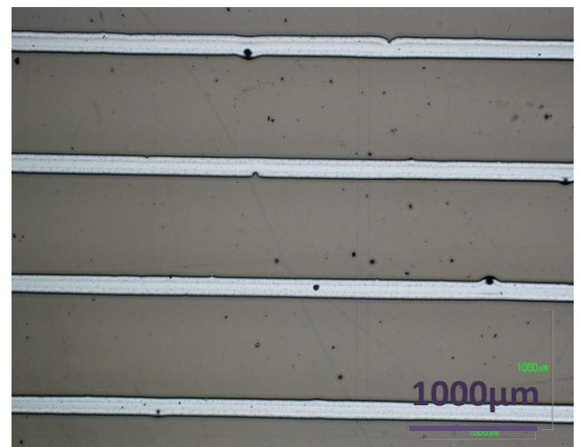
Fig 8.4.: Ag ink lines printed in Ormostamp O 2 plasma treated
