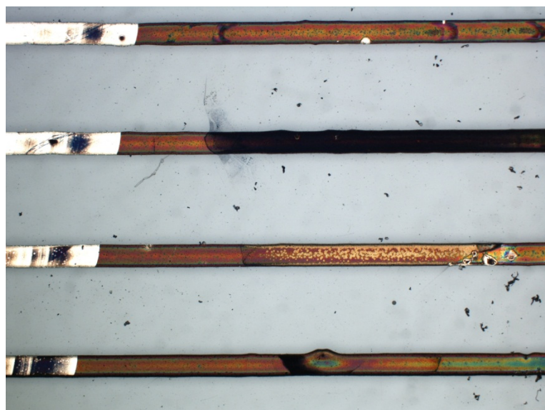
Fig 21: Ag/AgCl lines electrode after usage
