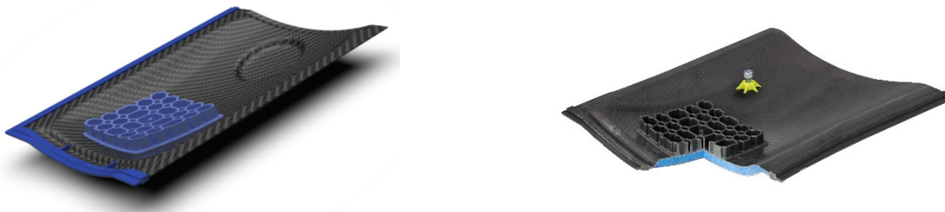
Fig. 4: Demonstration part “Functionalized 3D-Sandwich with bead foam core” (CAD-view on the left and realized component on the right).
