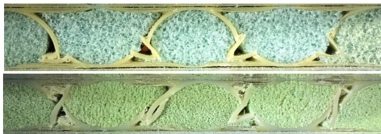
Fig. 2: Typical failure of GFRP samples for C40GF3 and C130GF5.
