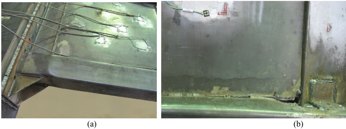
Fig. 3: Buckling of the specimen after the test.
