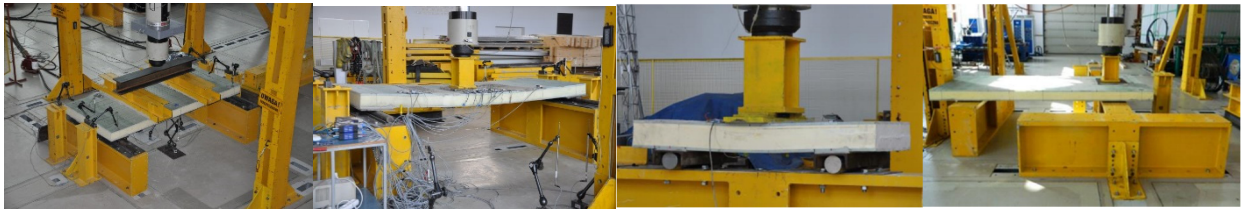
Fig. 2: Loading schemes of panel specimens: scheme 1 to scheme 4 from left to right.
