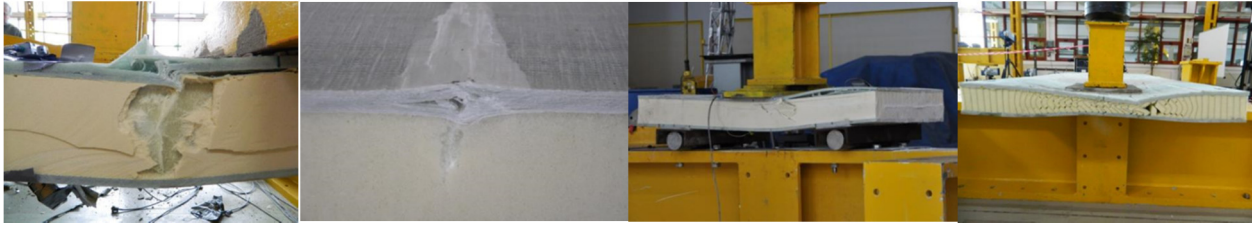
Fig. 4: Failure modes in particular loading schemes: scheme 1 to scheme 4 from left to right.
