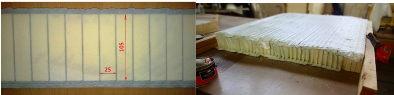
Fig. 1: Sandwich panel configuration (left) and panel prepared for VARTM.
