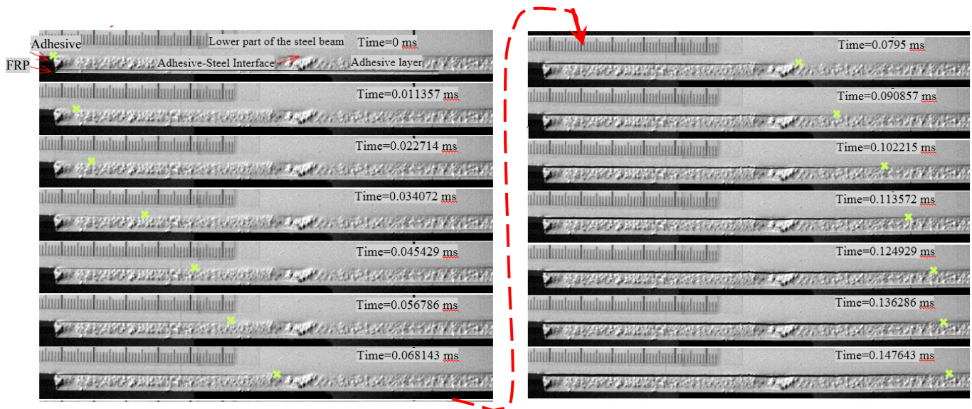
Fig. 2: Evolution of the interfacial debonding crack in time – experimental results (adapted from Mulian and Rabinovitch [3]).
