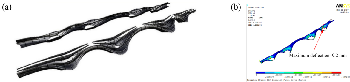
Fig. 3: FRP curved sandwich panels: (a) the groups and divisions; (b) the displacement of FEA results of bottom part.
