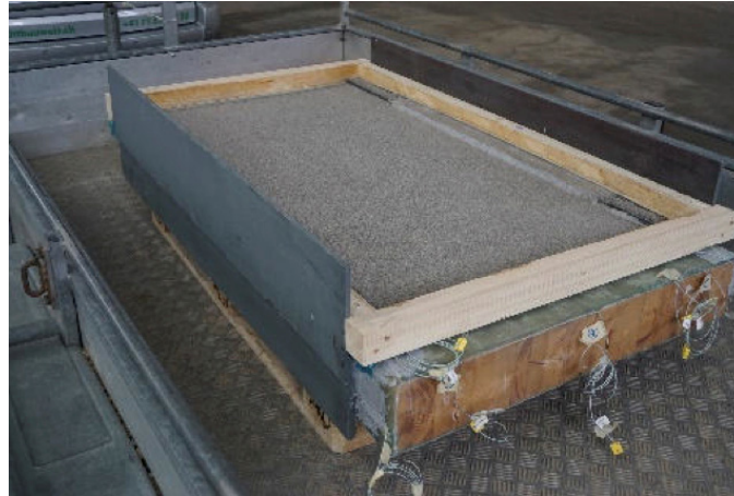
Fig. 2: Sample of the first preliminary test before asphaltting.
