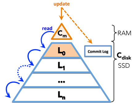
Figure 1: High-level view of a typical LSM KV store.
