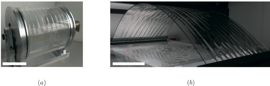
FIGURE 2. (a) Cylindrical substrate formed by a PMMA cylinder of radius R = 8.6 cm and length L_z = 15 cm partially filled with silicone oil. The axis of the cylinder is mounted on a motor which can reach 100 rpm for coating purpose. (b) Curved PMMA plate of 500 \times 200 \times 4 mm clamped at its extremities to prescribe the desired substrate curvature. The thin film of silicone oil is applied with a film applicator prior to deforming the plate. Scale bars correspond to 10 cm. Rivulets are visible on both figures.
