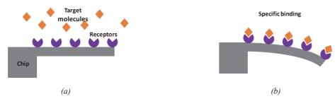
Figure 1.4: Working principle of a static mode biosensor. Binding of target molecules induces a surface stress, which leads to a quasi-static deflection of the cantilever. This bending can be measured with optical or electrical displacement detection methods.
