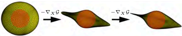
Figure 4. Minimizing the drag of the initially spherical surface under the constraint it must contain the smaller red sphere.
